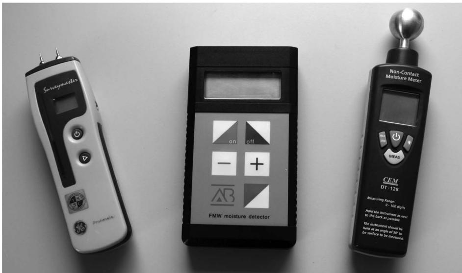
**Figure 1.** Photograph of each of the meters used in this experiment, from left to right: Protimeter, FMW-T and CEM.
